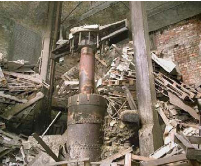
Fig 4.10.2: The hydraulic accumulator
